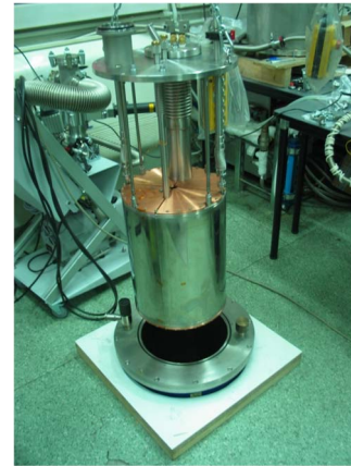
Fig. 5. Complete insert ready to be installed in cryostat.
