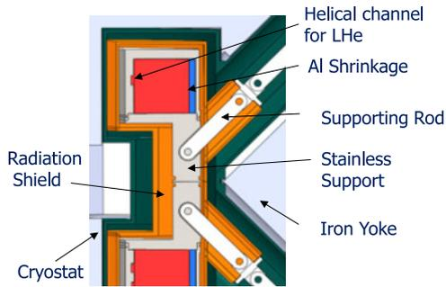
Fig. 2. Coil, cryostat and support structure cross section.
