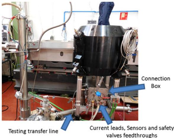
Fig. 5. Cyclotron magnet and transfer line for thermal characterization using external cryogenes from a Dewar
