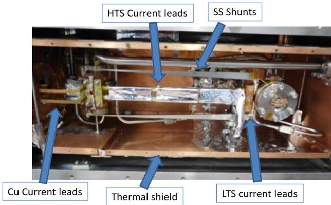
Fig. 3. Connection box assembly and its main components.
