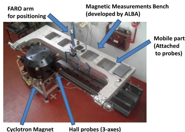
Fig. 1. Cyclotron magnet, magnetic test bench and alignment system for magnetic characterization.
